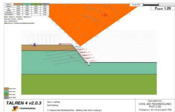
Fig4: Stability analysis for Retaining wall
