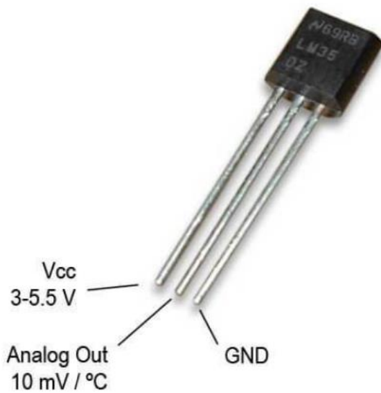
Fig 3: Pin Diagram Of LM35
