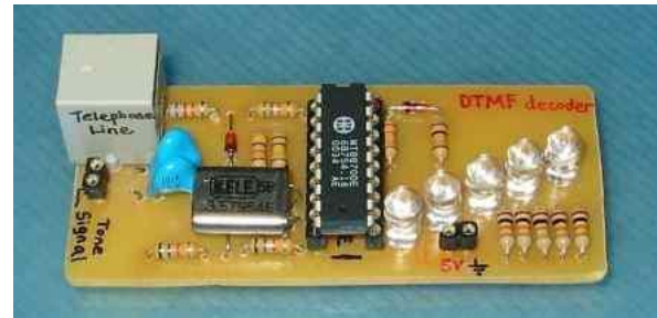
Fig. 1: DTMF Decoder (MT8870)
