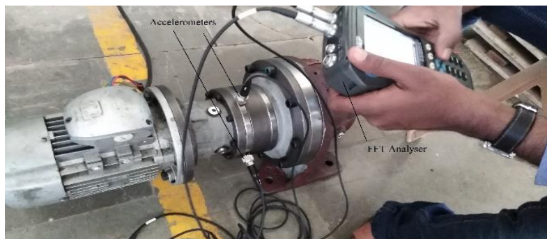
Figure 2 Test ring with FFT analyzer
