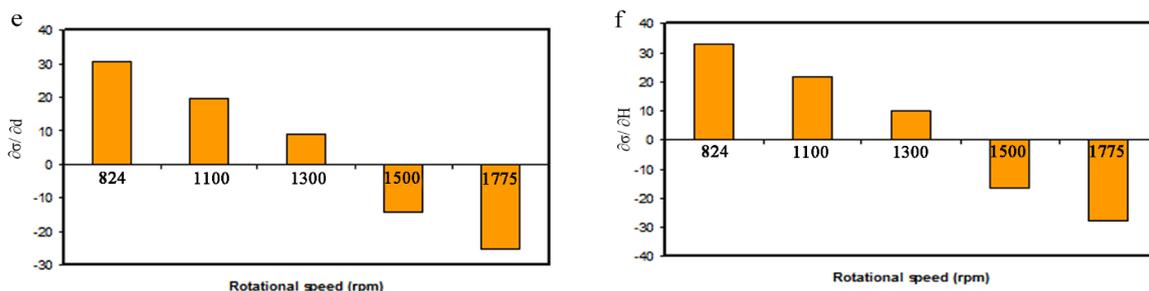
**Fig. 4** Sensitivity analysis results: (a). Rotational speed (rpm); (b). Welding speed (mm/min); (c). Axial force (kN); (d). Shoulder diameter (mm); (e). Pin diameter (mm); (f). Tool hardness (Hv);
