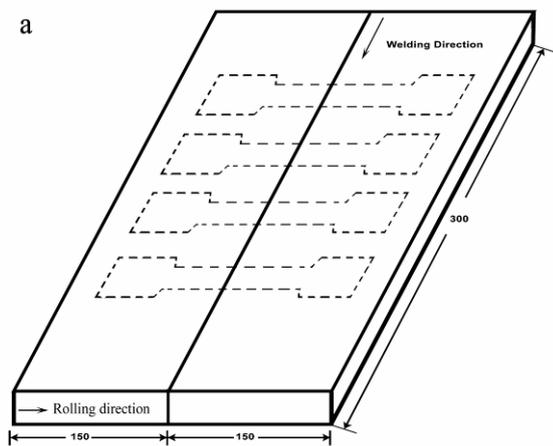
(a) Joint dimensions (in 'mm')
