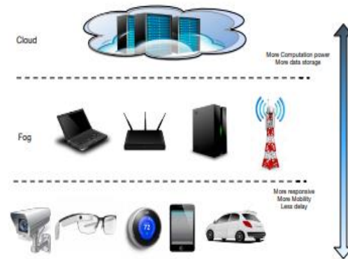
Fig. 1. An example of fog/cloud architecture
