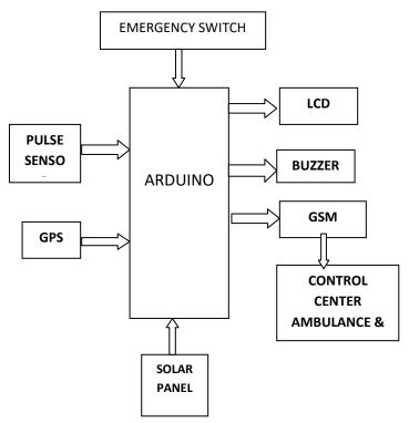
This block diagram consists of Arduino, LCD, Buzzer, GSM, GPS, pulse sensor, solar panel, and emergency switch.
