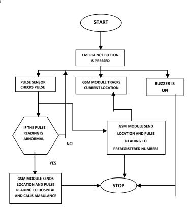
In case if the pulse reading also goes abnormal then the Arduino command the GSM module to send the pulse reading by SMS and to call the ambulance so that the immediate medical help can be provided .
