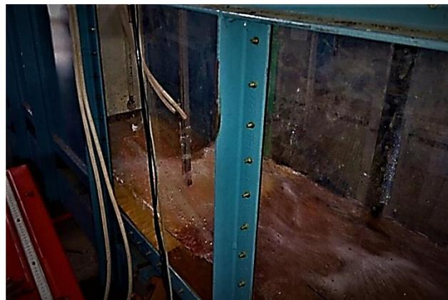
Fig.7 Hydraulic jump on the right angle triangle corrugated bed
