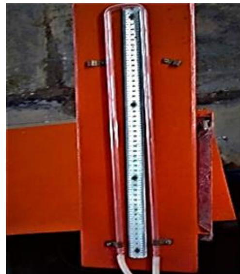
**Fig.4 Inclined manometer**
