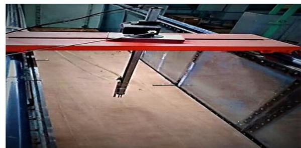
**Fig.5 Point gauge mounted on the moving trolley**
