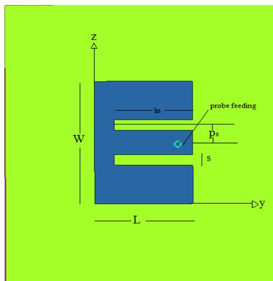
Figure 1: Top view of E-shaped patch antenna
