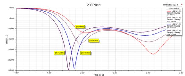
Figure 5: Variation of return loss with frequency for different slot positions at  $s=6$  mm and  $l_n=40$  mm
