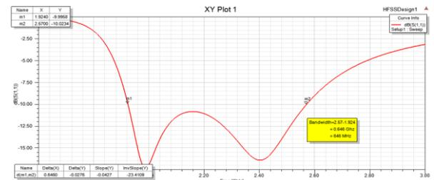
Figure 6: Variation of return loss with frequency for  $l_n = 40$ mm,  $s=6$  mm and  $p_n=40$  mm
