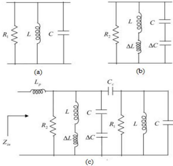
Figure 2: (a) Equivalent circuit of centre wing. (b) Equivalent circuit of side wing. (c) Complete equivalent circuit of E-shaped patch antenna
