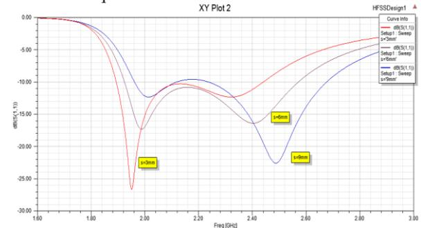
Figure 4: Variation of return loss with frequency for different slot widths at  $p_n=10$  mm and  $l_n=40$  mm
