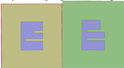
(a) Unequal slot lengths (b) Unequal side wings
