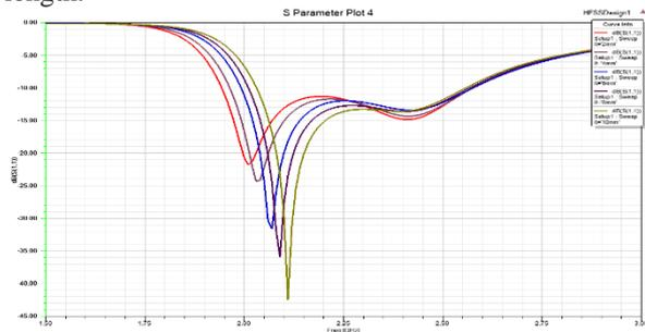
Figure 10: Return loss characteristics for various slot lengths
