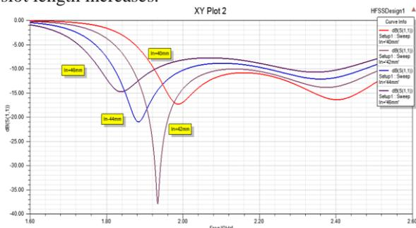
Figure 3: Variation of return loss with frequency for different slot length at  $p_n=10$  mm and  $s=6$  mm
