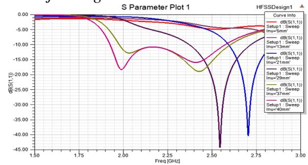
Figure 11: Return loss characteristics for various side wing lengths
