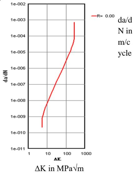
Figure 34: Crack growth rate for thickness 27.2mm.
