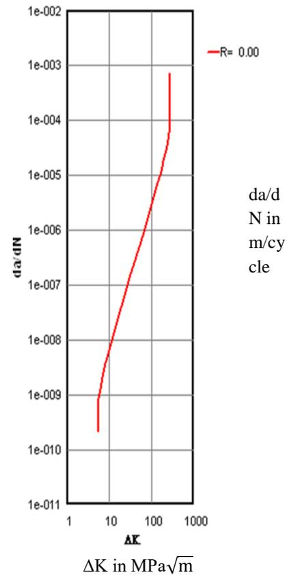
**Figure 32: Crack growth rate for pressure 22MPa.**
