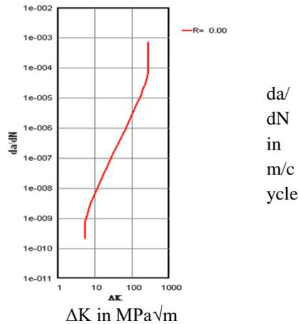
Figure 38: Crack growth rate for thickness 17.2mm.
