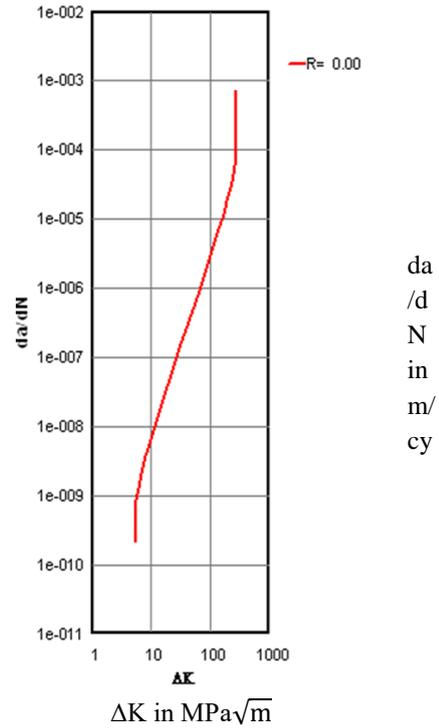
Figure 28: Crack growth rate for pressure 14MPa.
