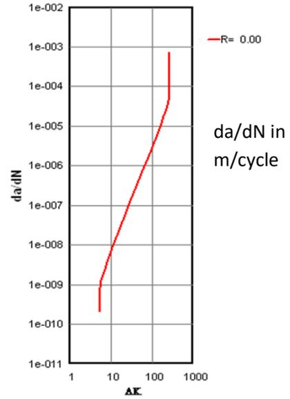
Figure: 54 Crack growth rate for thickness 22.2mm.
