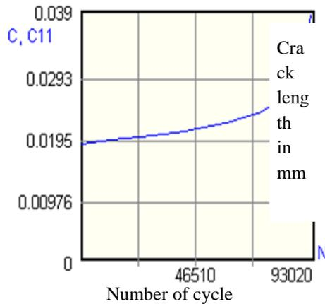
Figure 16: Crack length versus number of cycle.
