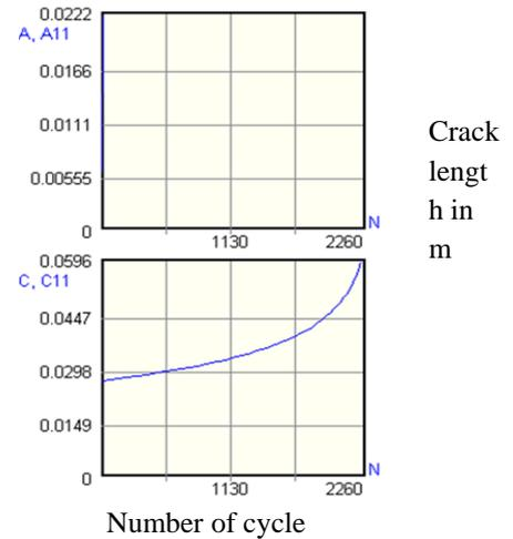
Figure 35: Crack length versus number of cycle for thickness of 22.2mm.
