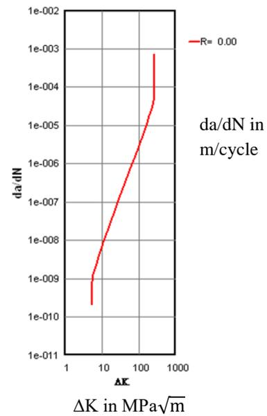
Figure: 58 Crack growth rate for thickness 17.2mm.
