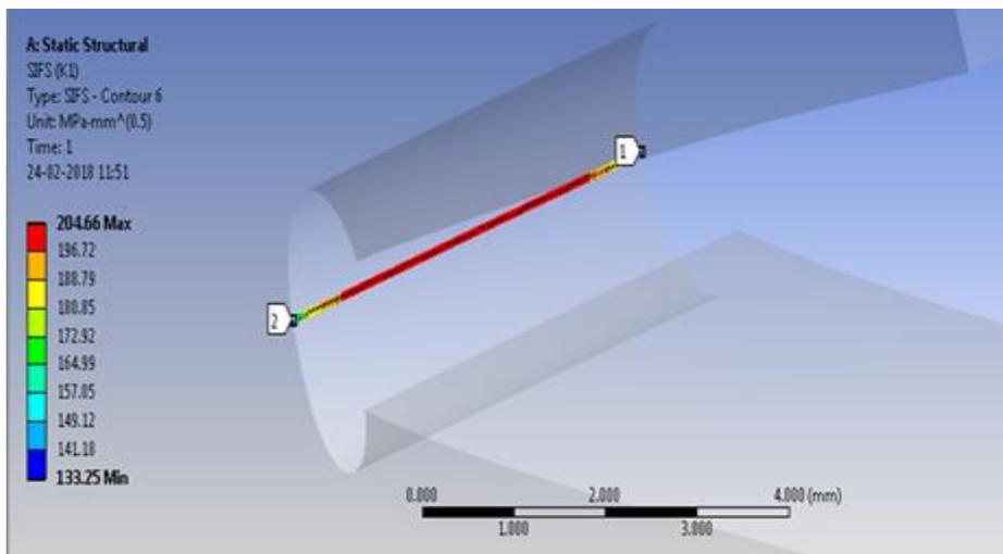
Figure 4: Stress intensity factor of compact tension specimen.
