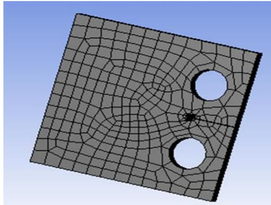
Figure 2: Meshed model of compact tension specimen.
