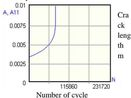
**Figure 10: Crack length along thickness versus number of cycles.**
