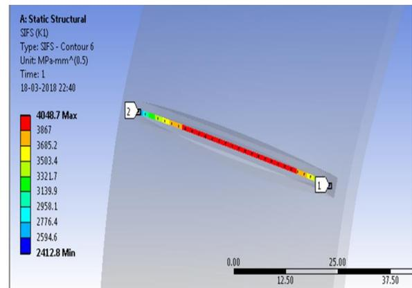
Figure 24: Stress intensity factor of pressure vessel.
