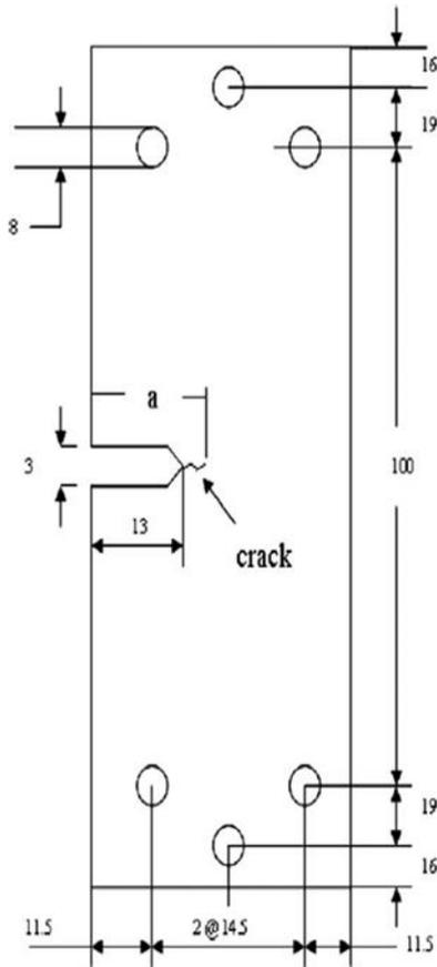
Figure 13: Geometry of single edge notch crack.
