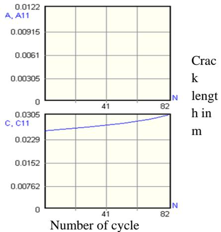
Figure 29: Crack length verses number of cycle for pressure of 18MPa.
