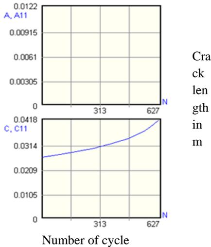
Figure 27: Crack length verses number of cycle for pressure of 14MPa.
