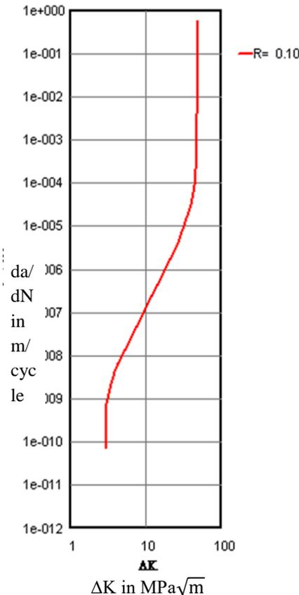
Figure6: Crack growth rate.
