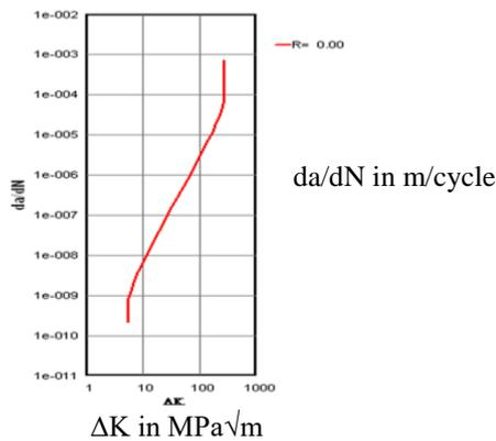
Figure 40: Crack growth rate for thickness 12.2mm.
