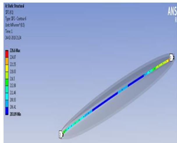
Figure 9: Stress intensity factor of semi elliptical specimen.
