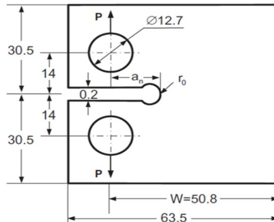
Figure 1: Dimension of compact tension specimen.
