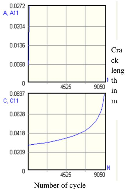
Figure 33: Crack length versus number of cycle for thickness of 27.2mm.
