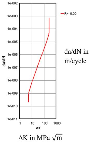
Figure: 52 Crack growth rate for thickness 27.2mm.
