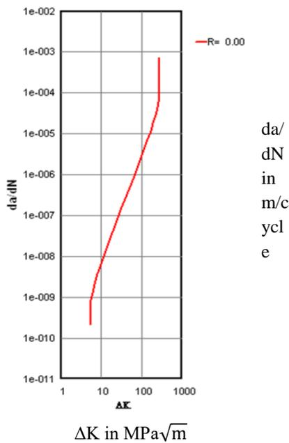
**Figure 30: Crack growth rate for pressure 18MPa.**
