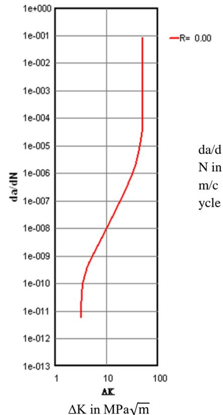
**Figure 12: Crack growth rate.**
