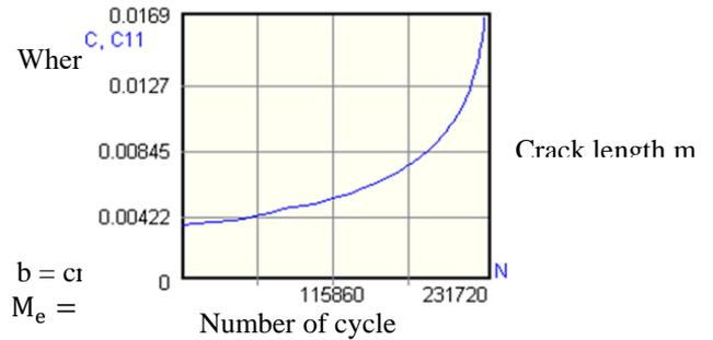
**Figure 11: Crack length along width versus number of cycles.**
