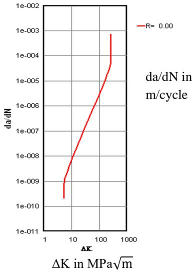
Figure: 46 Crack growth rate for pressure 14MPa.
