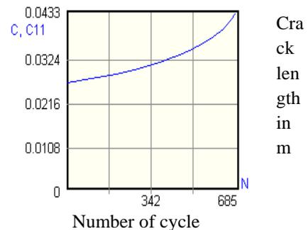
Figure: 45 Crack length along width verses number of cycle for pressure 14MPa.
