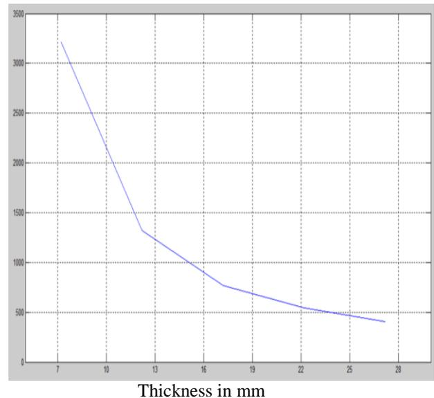
Figure 26: Stress intensity factor verses thickness.
