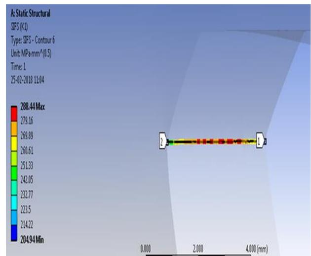
Figure 15: Stress intensity factor of single edge notch crack specimen.
