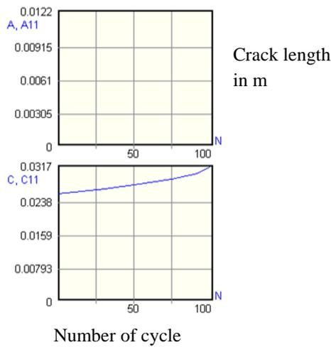
Figure: 47 Crack length for pressure 18MPa.
