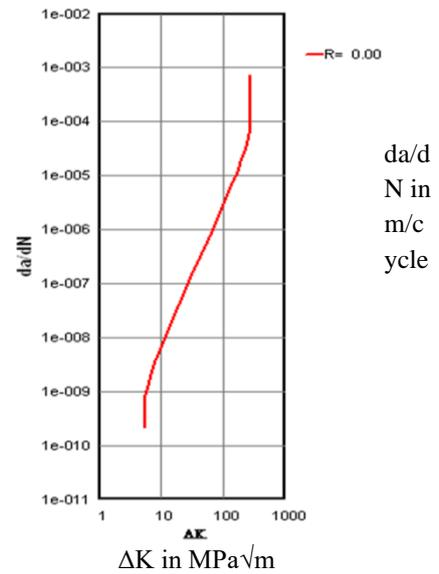
Figure 36: Crack growth rate for thickness 22.2mm.
