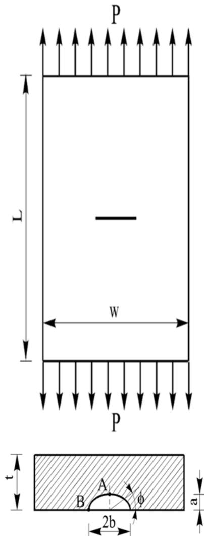
Figure 7: Geometry of semi elliptical crack.
