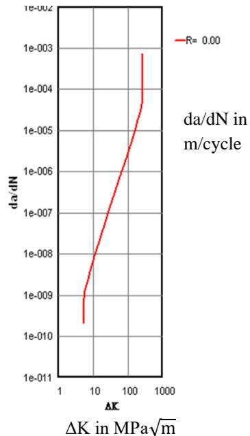
Figure: 50 Crack growth rate for pressure 22MPa.
