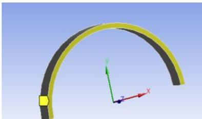
Figure 22: Restricting along Z direction.
