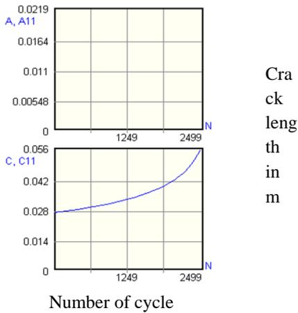
Figure: 53 Crack length for thickness 22.2mm.
