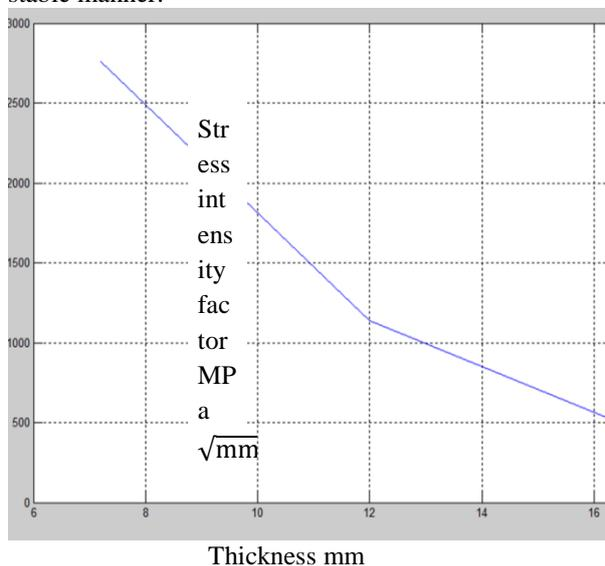
Figure: 43 Stress intensity factor verses thickness.
