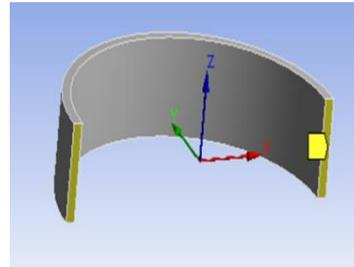
Figure 23: Restricting along X direction.
