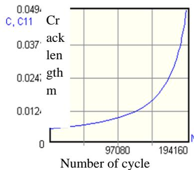
Figure 5; Crack length versus number of cycles.
