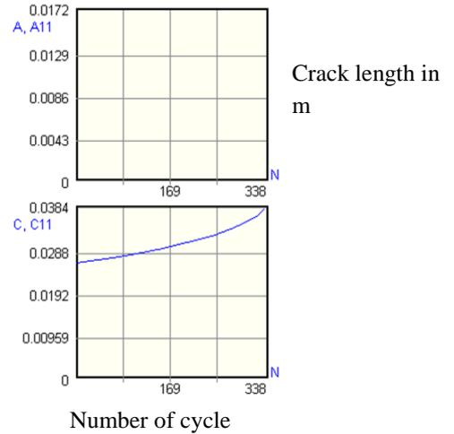
Figure: 55 Crack length for thickness 17.2mm.
