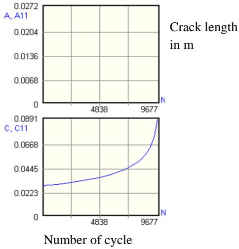
Figure: 51 Crack length for thickness 27.2mm.
