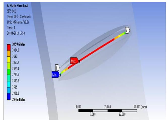
Figure 41: Stress intensity factor of internal axial crack in pressure vessel.
