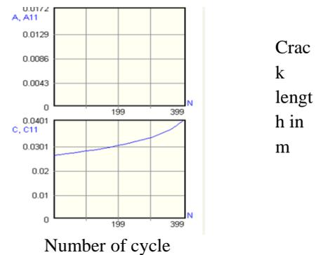
Figure 37: Crack length versus number of cycle for thickness of 17.2mm.
