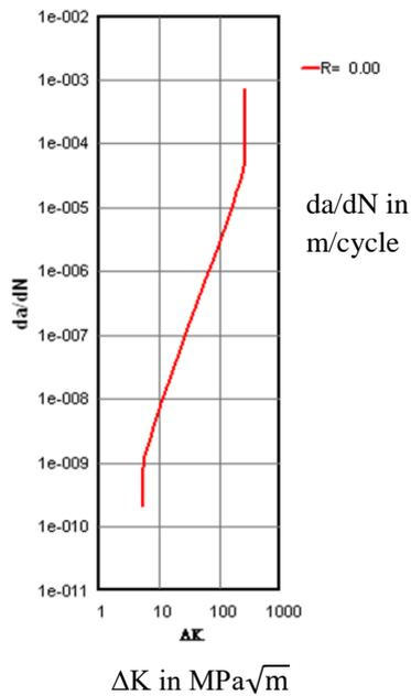
Figure: 56 Crack growth rate for thickness 17.2mm.
