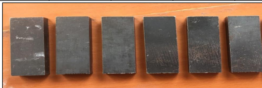
Figure 1 Standard test specimens of size 75x25x10mm
