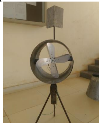
Figure 2. Experimental setup of bare wind turbine
