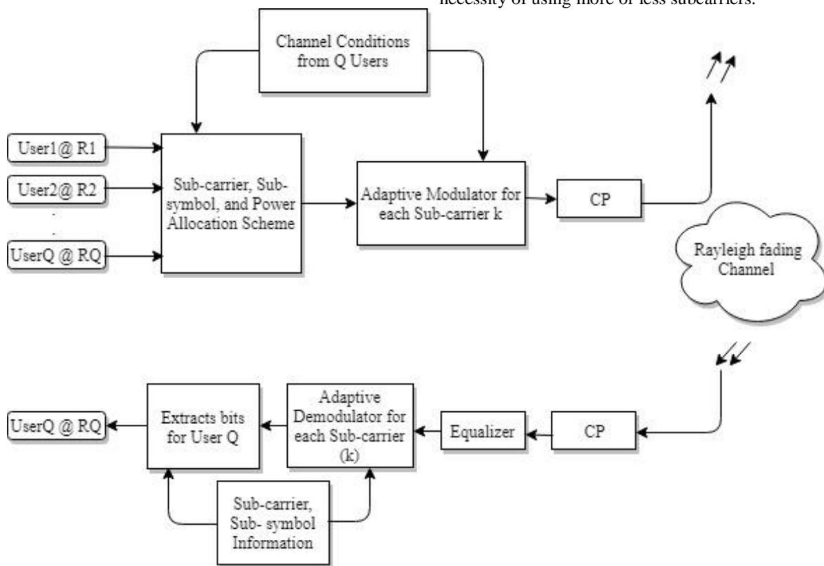
Figure3: Multi-user GFDM with adaptive allocation
