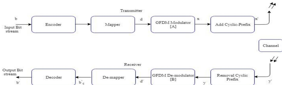
Figure2: Block diagram of GFDM
