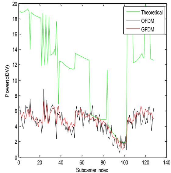
Figure 8: Power (dBW) versus different subcarriers using OFDM and GFDM
