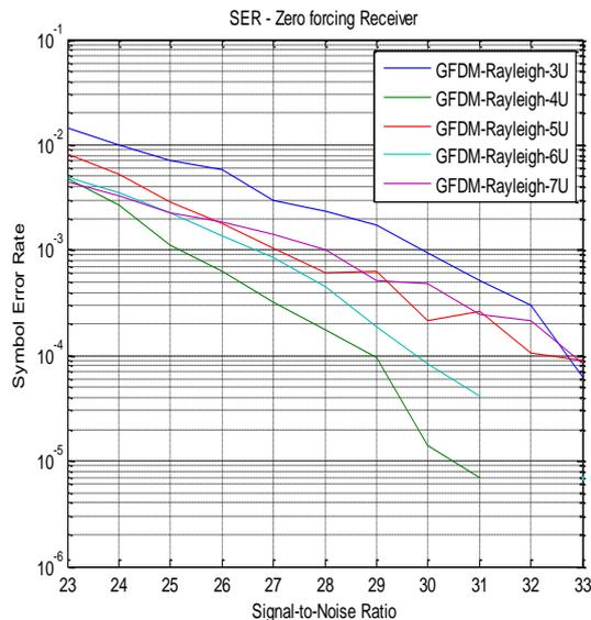
Figure 7: Signal to Noise ratio versus SER for different users
