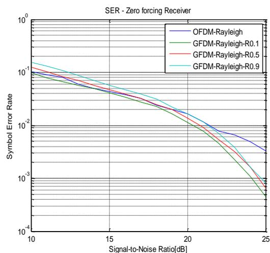
Figure 6: Signal to Noise ratio versus SER for different Roll off factors
