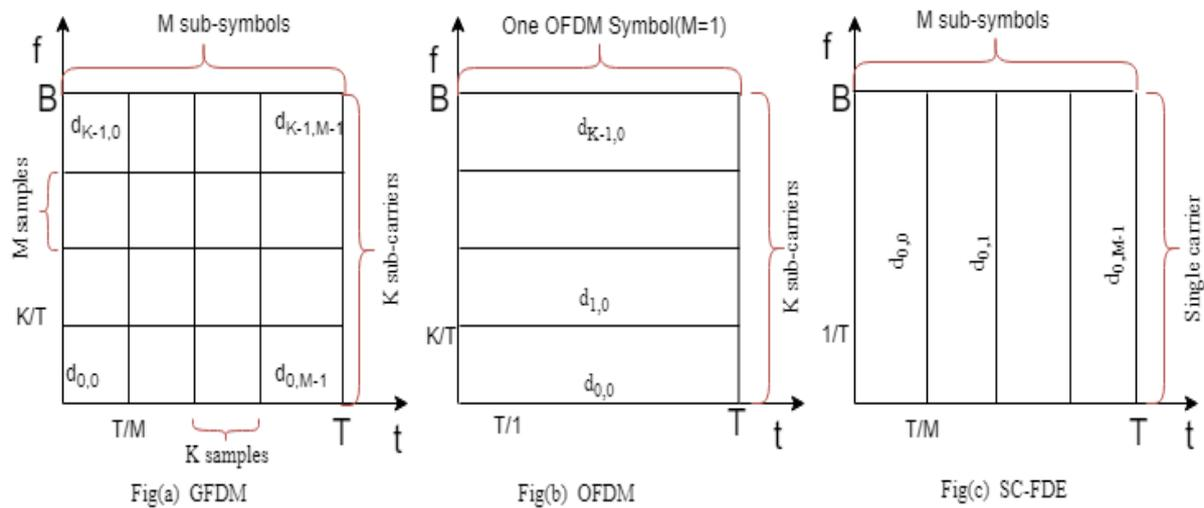
Figure1: Concept of GFDM by setting number of sub carriers and sub symbols
