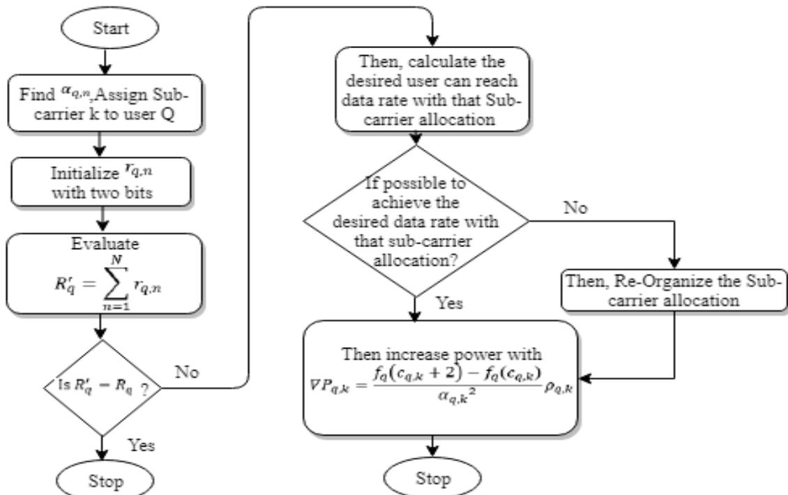
Figure4: Flow chart for Multi-user GFDM with adaptive allocation
