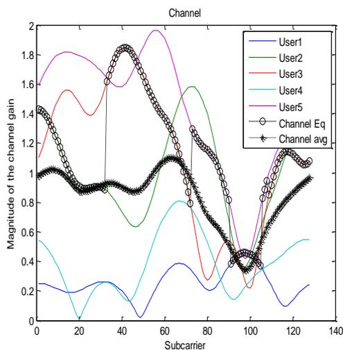
Figure 5: Magnitude of the channel gain varying with number of sub-carriers
