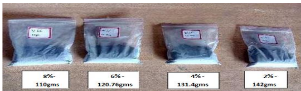
Fig. 3 - Weighed and sorted SiC particles as per the requirement
