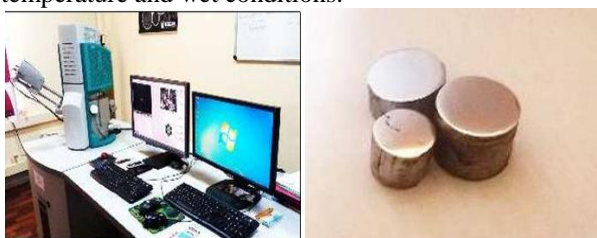
Fig. 14 - SEM equipment & Mirror polished specimen ready for SEM analysis
