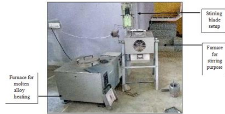
Fig. 6 - Experimental setup of stir casting
