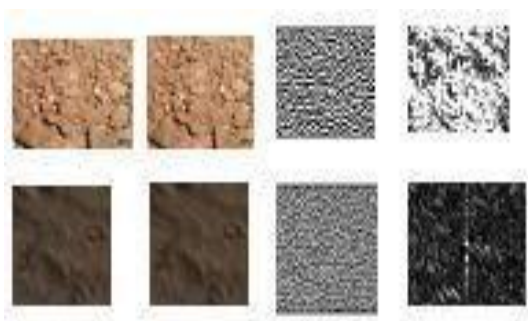
Fig 2 a) original image of clay soil b) color quantized c) S5S5 law mask filter d) Gabor filter e) original image law masks of alluvial soil f) color quantized alluvial soil g) S5S5 h) Gabor filter alluvial soil
