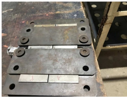
(a) Clamping of the work piece (b) CO 2 laser beam welding set up
