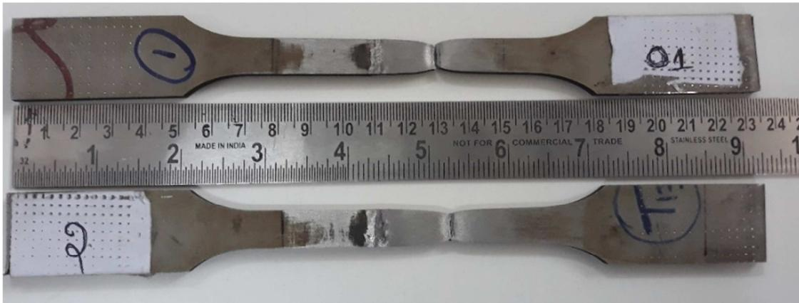
Fig 8: Tensile strength specimens (a) Gauge length of the weldment (b) failure of weld tensile samples
