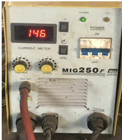
Fig. No. 1 DC output power source
