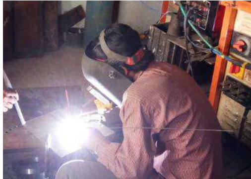
Fig 4- Welding of SS sheet
