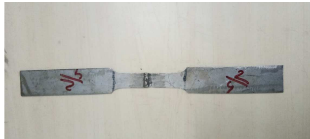
Fig 6- Tensile specimens of SS-210 & 310
