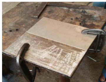
Fig-2 Welding of SS-310 and ss-202
