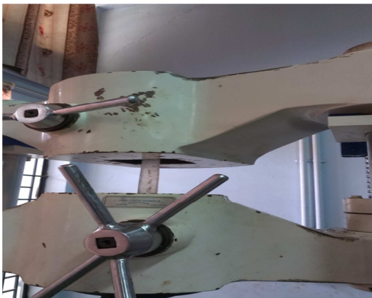
Fig 3: Tensile test specimen loaded in UTM
