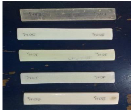
Fig 2: Bending test specimens
