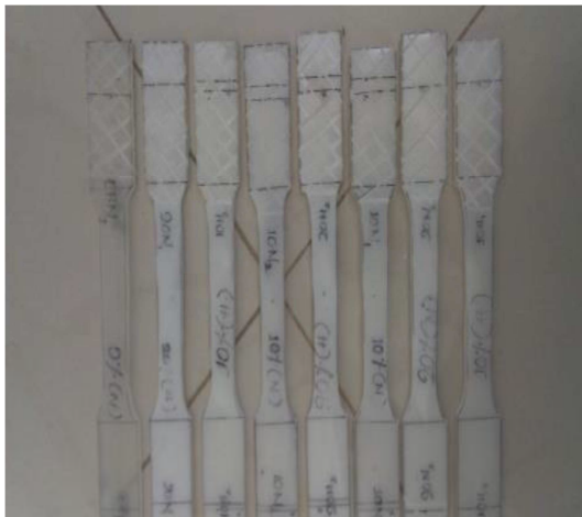
Fig 1: Tensile test specimens
