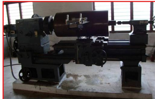
Figure 2: Filament Winding Machine
