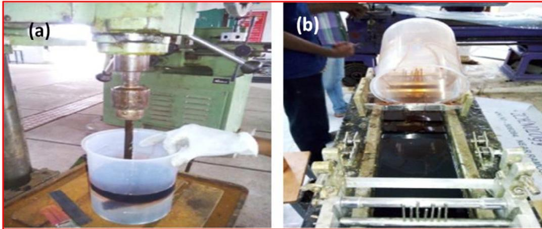
Figure 1: (a) Resin mixing and (b) Creel Stand
