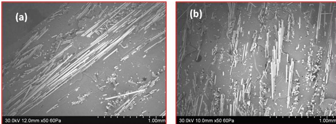
Figure 4: Fractographs of glass fiber reinforced epoxy matrix composite
