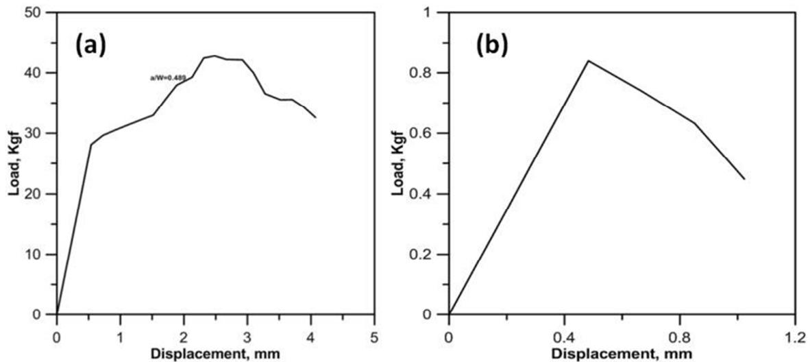
Figure 3: Load Vs Displacement data of (a) Longitudinal (b) Transverse composite specimens
