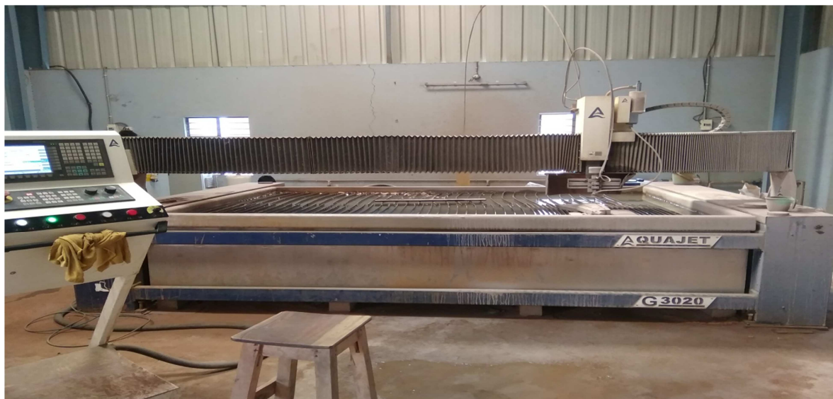
Fig :2. Abrasive Water jet Machining setup used for the Experiment of EN-8
