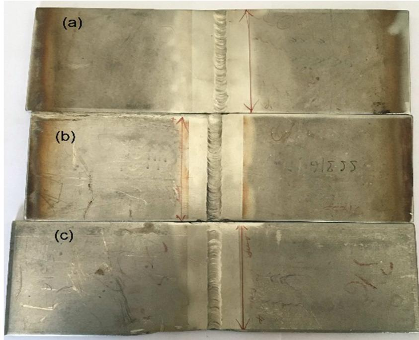
**Fig. 2.** Dissimilar welded joints of AISI 316 and Monel 400
