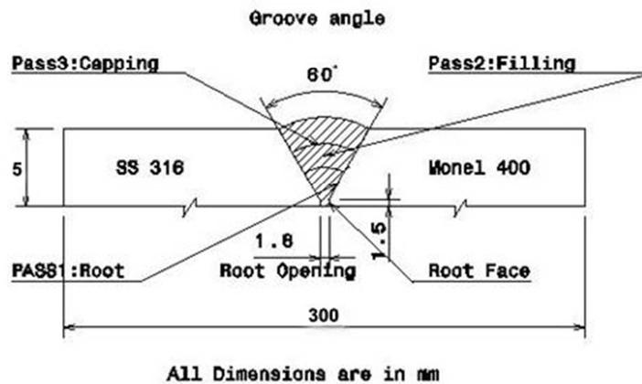
**Fig. 1.** Schematic diagram of weld groove design
