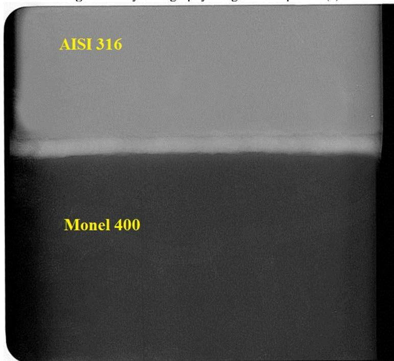
**Fig. 4.** X-Ray radiography image of Sample ID-(b)
