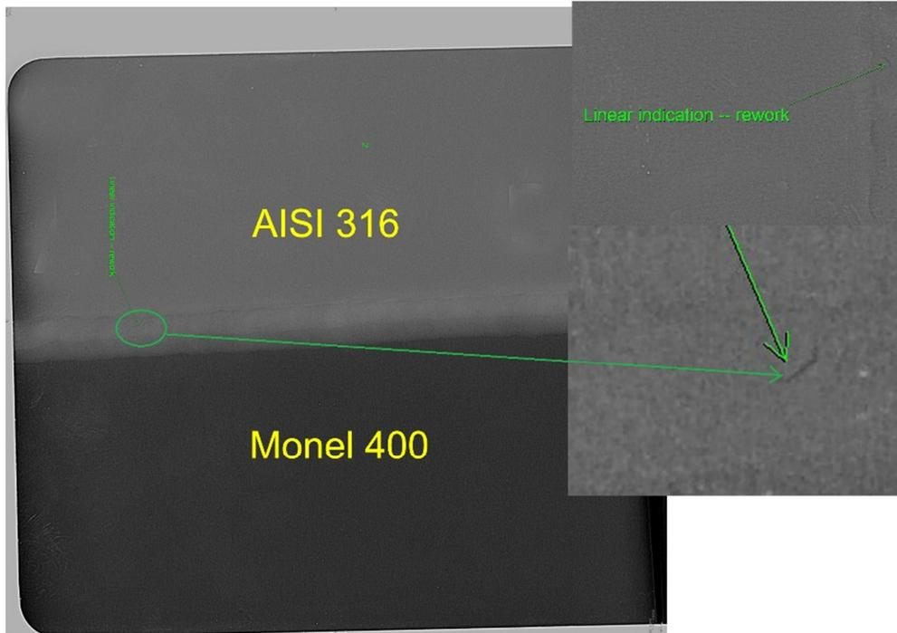
**Fig. 3.** X-Ray radiography image of Sample ID-(a)
