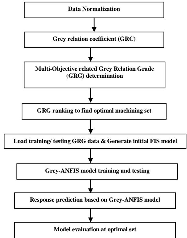
Fig. 2. Schematic diagram of the proposed approach
