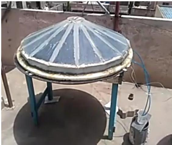
Fig 2. Experimental setup of conical solar still.
