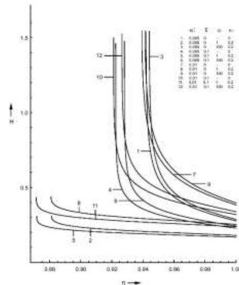
Figure 2(d): Variation of magnetic field in the region behind the shock front.
