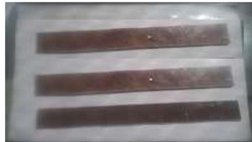
Figure 2: work pieces obtained using hand lay-up process
