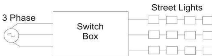
Fig. 5. Block Diagram of Case Study 2
