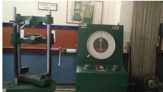
Fig 6:- Universal Testing Machine
