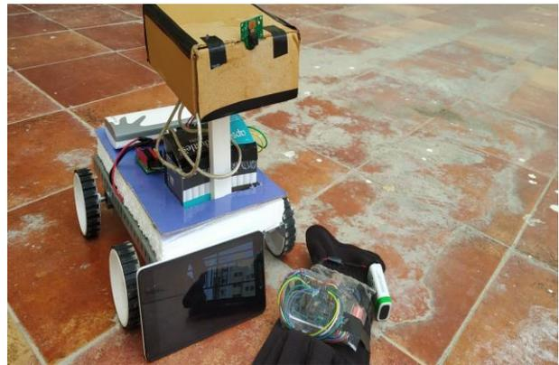
Figure 11. Over all view of the model which gives us Virtual Telepresence and controlling through hand gestures.
