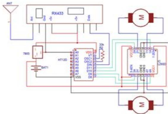
Figure 3. Receiver Circuit
