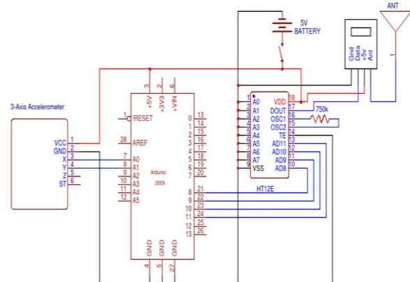
Figure 2. Transmitter Circuit
