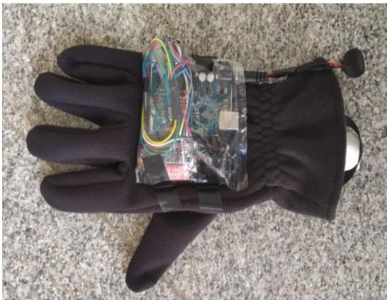
Figure 9. Transmitter Design in which the accelerometer sensors the movement and feeds signals to the Arduino UNO microcontroller.
