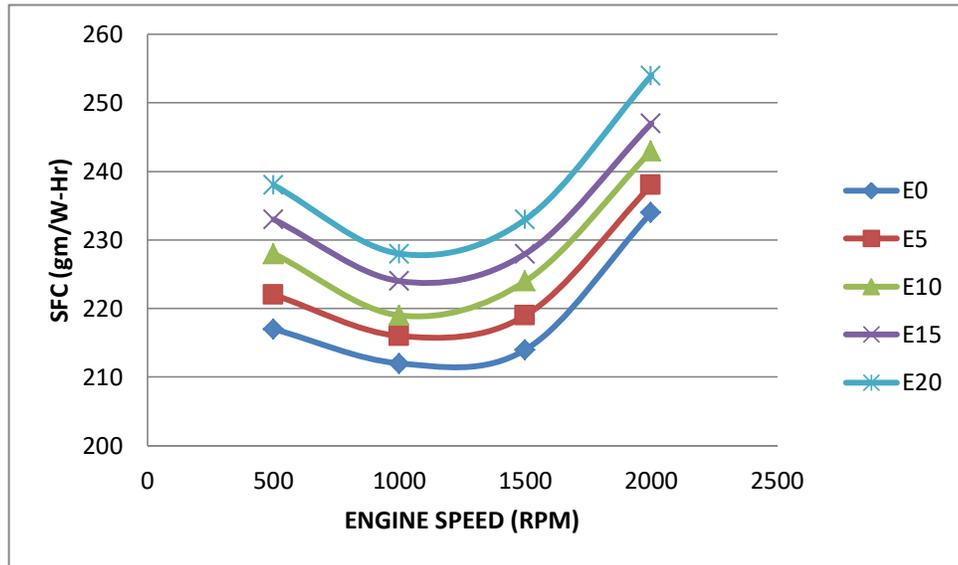
Graph 4.3 Variation of brake specific fuel consumption and engine speeds for different blending ratios
