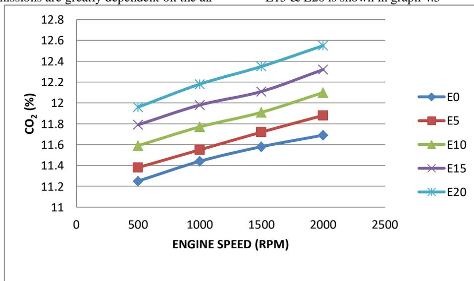
Graph 4.5 Variation of carbon dioxide and engine speeds for different blending ratios
