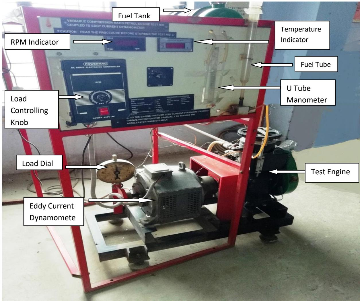
Fig. 1 Experimental set-up
