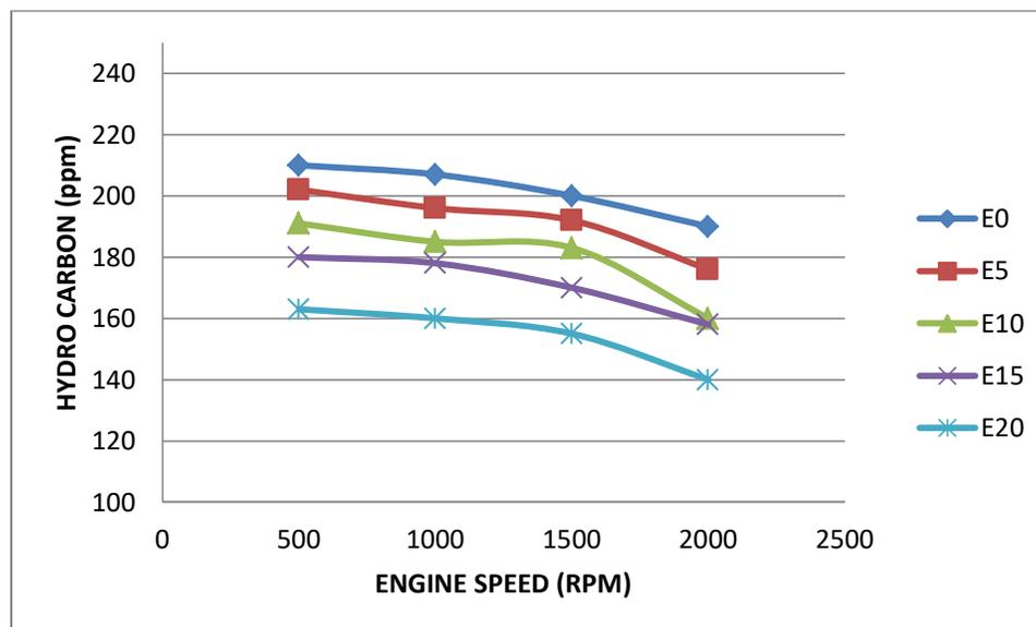
Graph 4.6 Variation of hydrocarbon and engine speeds for different blending ratios
