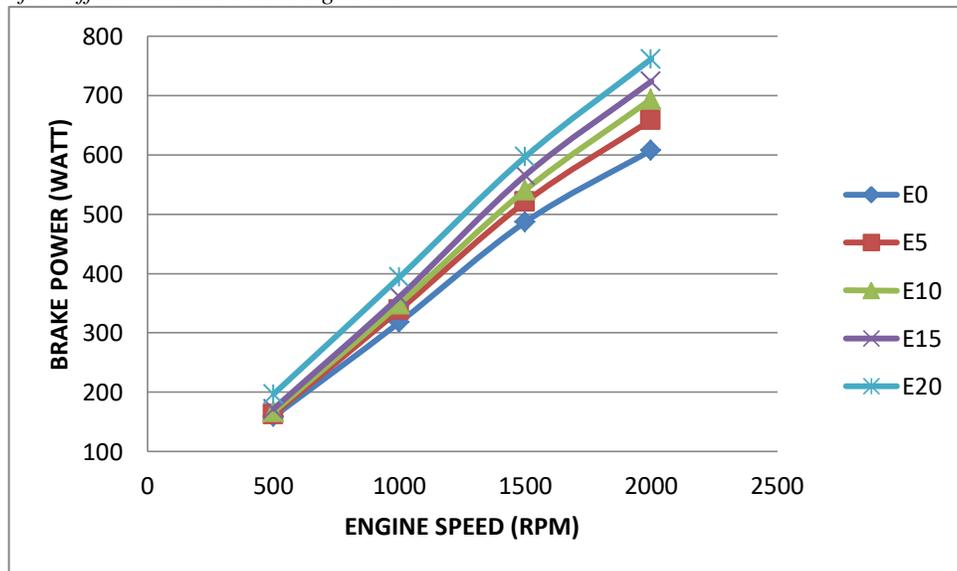
Graph 4.2 Variation of brake power and engine speeds for different blending ratios
