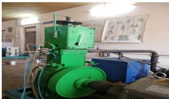
Fig.1, Computerized VCR engine test rig
