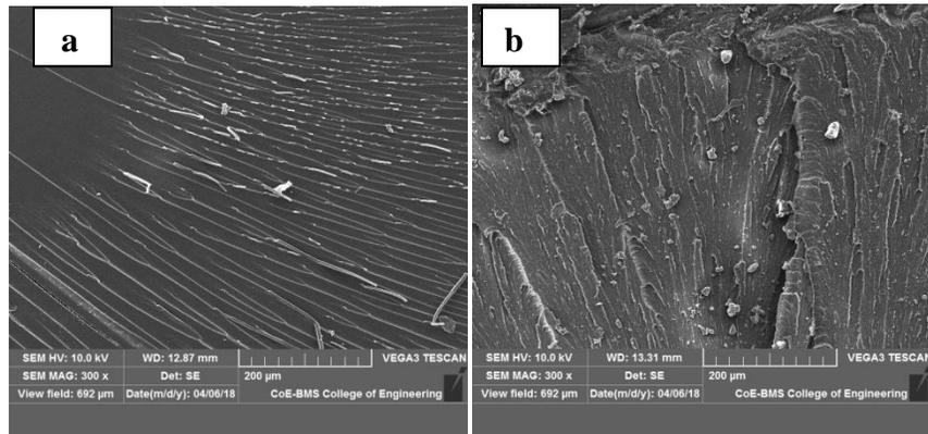
**Fig1.**Scanning electron micrographs showing fractured surface of (a) pure epoxy, (b) for samples containing 2 weight% PMMA.
