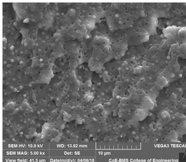
**Fig 3.** Magnified view of 6 wt % PMMA
