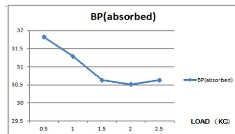
Fig. 10: Brake Power Vs Load
