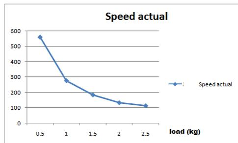
Fig. 11: Speed Vs Load
