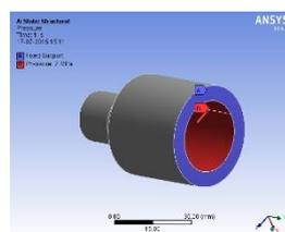
Fig. 4: Fixed support & Load Application on Thruster Body
