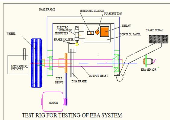
Fig. 1: Schematics of test rig of EBA system
