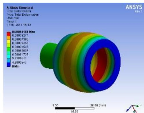
Fig. 6 : Total Deformation of Thruster Body
