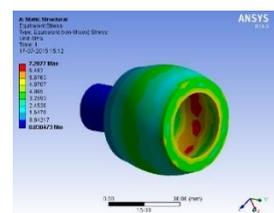
Fig. 5: Equivalent Stress (Von – Mises) of Thruster Body
