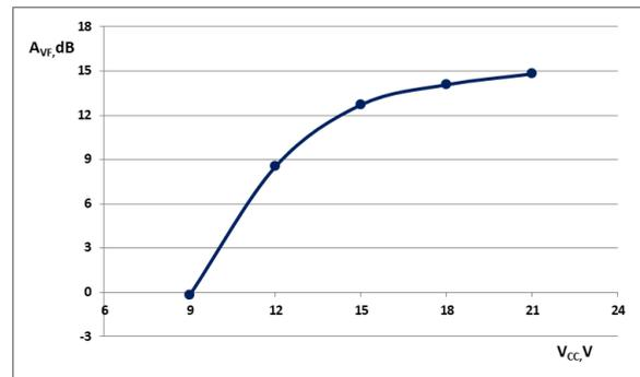
Fig.2. Voltage Gain with Negative Feedback versus Supply Voltage for UBCT Cascode Amplifier
