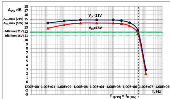
Fig.3. Frequency Response of UBCT Cascode Amplifier
