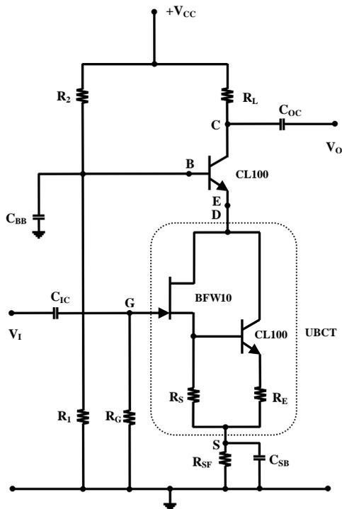
Fig.1. Circuit Design of UBCT Cascode Amplifier
