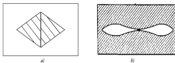
Figure 4. a) Bicone antenna, b) Conformal reverse bicone antenna (magnetic antenna)
