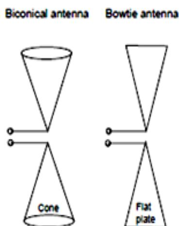
Fig 2: Few wideband Bowtie antenna types
