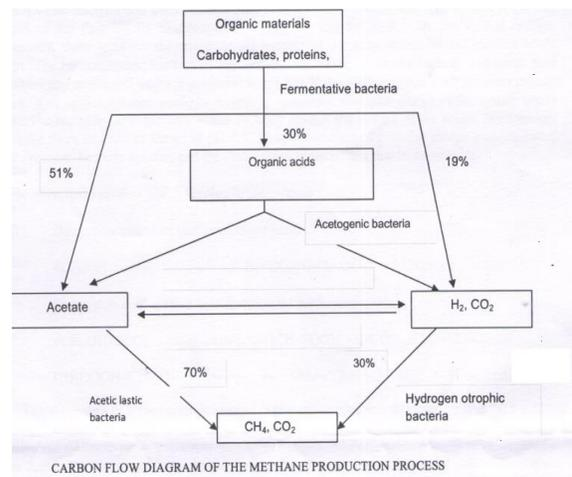
Figure 1. Flow chart of methane production
