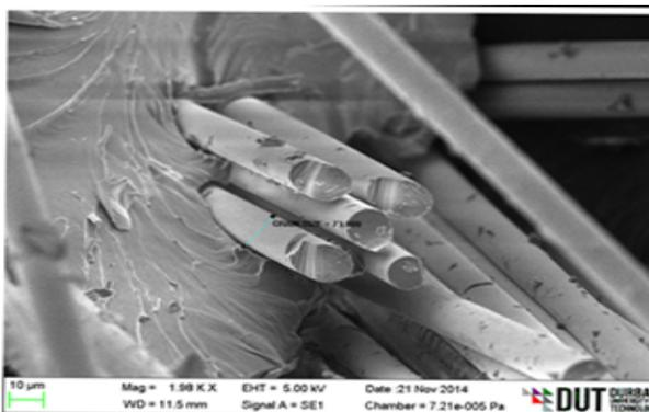
fig 8. Diameter of treated cow dung fiber
