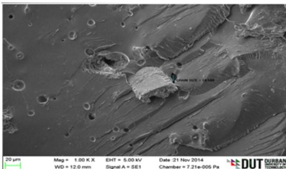
Fig 9. Void size of treated cow dung fiber composite
