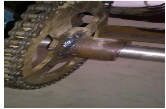
Fig 6: shaft with collar
