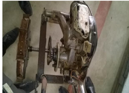
Fig 2: Scooter engine is placed on frame
