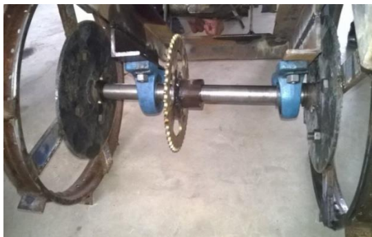
Fig 5: pillow bearing and shaft collar
