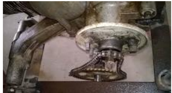
Fig 8: chain drive between cam shaft and sprocket
