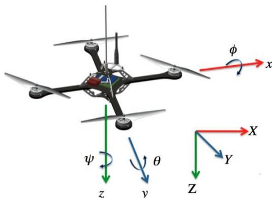
Fig. 1, Quadcopter dynamics and axes system
