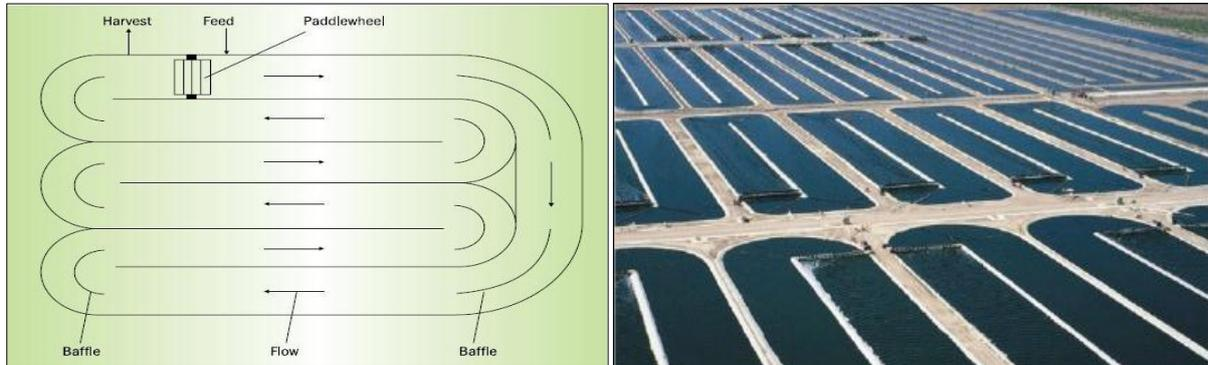
Fig.3- A raceway pond system
