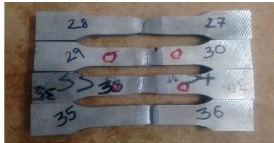
Fig. 5. Fractured specimens of weld joints formed from Hexagonal tip tool
