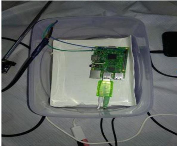
Fig9. Raspberry working as FM transmitter
