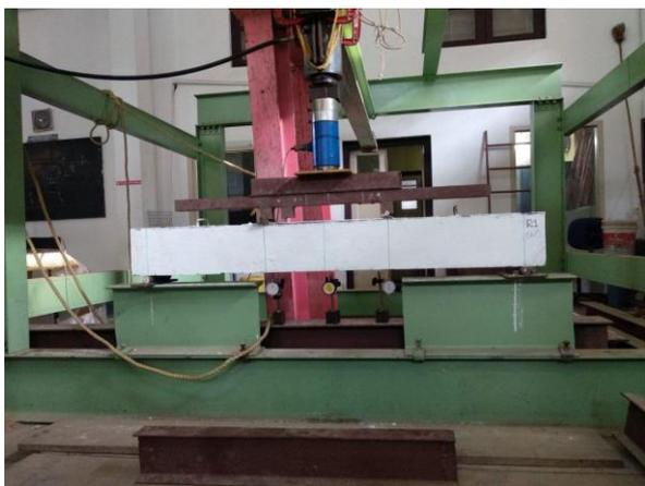
Fig.2. Flexural Test Setup
