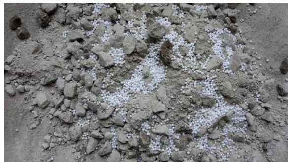
Fig. 4 mixing of aggregate, Fly ash and EPS
