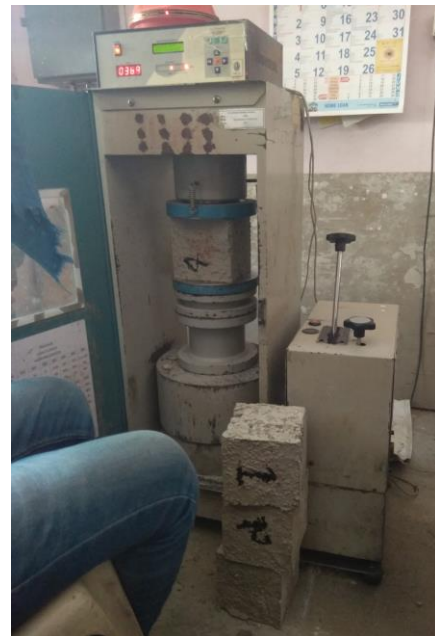
Fig. 7. Specimens at the time of compressive testing in CTM machine
