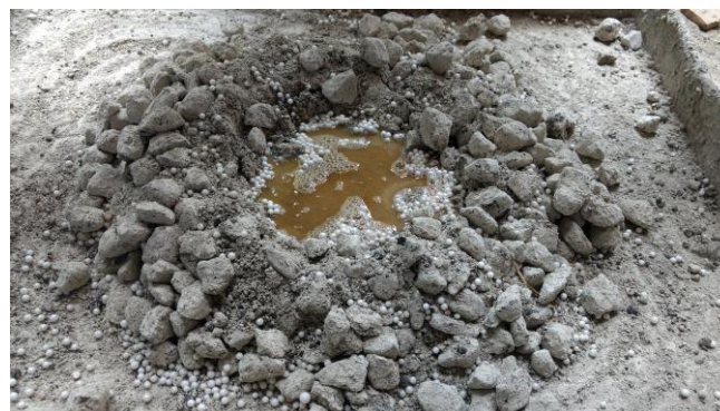
Fig. 5 mixing of all the ingredients of light weight geopolymer concrete
