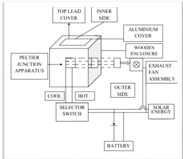
Fig.4: Block Diagram
