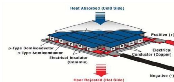
Fig.1: Peltier Structure
