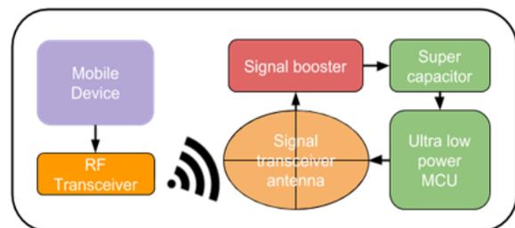
Figure 2: RF energy harvesting test bed
