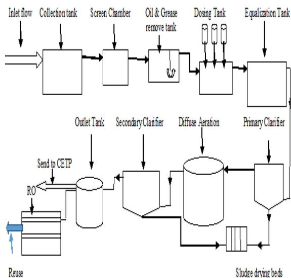
Figure 1- Flow Diagram of Textile Effluent Treatment Plant.
