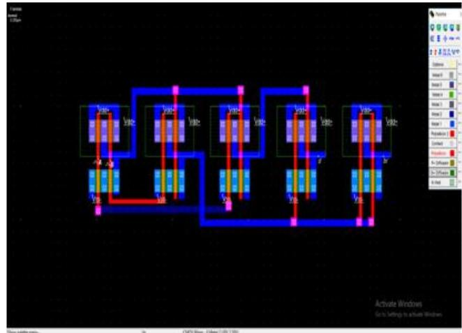
Fig.7. Semi custom layout of the half subtractor
