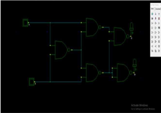
Fig.3. Schematic diagram of half subtractor
