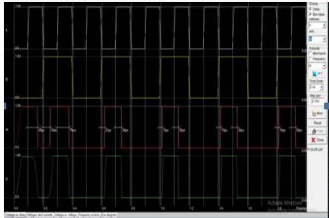
Fig.8. Output timing simulations of manual design
