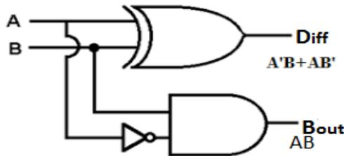
Fig.1. Conventional one bit half subtractor [2]
