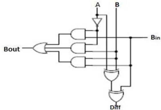
Fig.2. Conventional circuit of full subtractor
