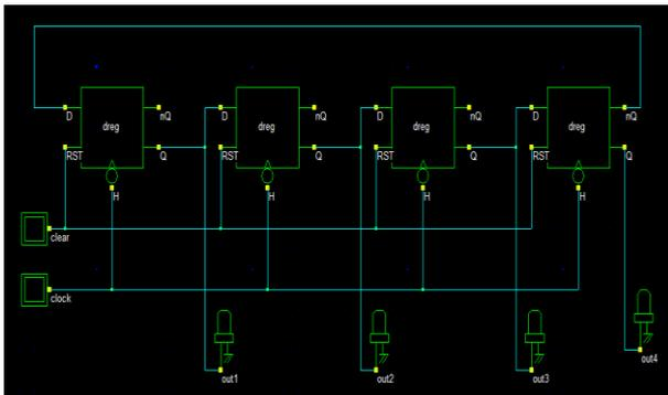
Fig.5. 4-Bit Johnson Ring Counter in DSCH
