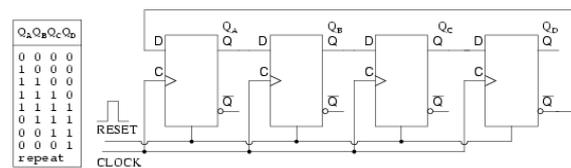
Fig.4. Four Bit Johnson Ring Counter
