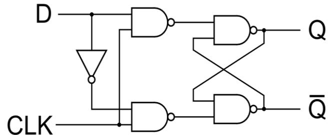
Fig.1. D flip-flop using NAND Gate
