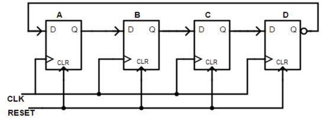
Fig.2. Synchronous Ring counter
