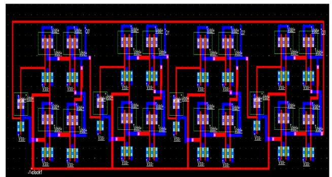
Fig.8.Semi-Custom Layout of 4- bit Johnson Ring Counter
