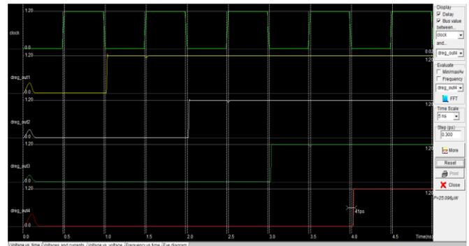
Fig.7. Auto Generated 4-bit Johnson ring counter output
